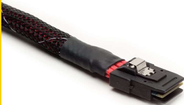
Multi-lane SFF-8087, SFF-8470, and M8 cables provide internal connectivity from the controller to drives or the backplane. Multi-lane SFF-8088 cables provide external connectivity from the controller to external enclosures.
